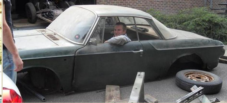
**What do you plan to do next?** I will finish the other side rocker panel first. Then I will put the body back onto the chassis so I can redraw the holes were the mounting screws go. I have to do it this because rust ate all the metal and it was impossible to measure from the existing holes.
