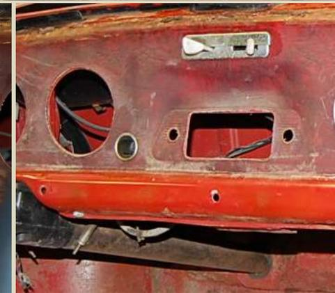
Once Thom made it to disassembling the instrument panel he discovered the previous owner had glued a vinyl covering over the Ruby Red dash. Another unpleasant discovery was the rust along the top-left edge underneath the upper dash pad and the mounting bolts (cast into the dash pad foam) had completely disintegrated.
