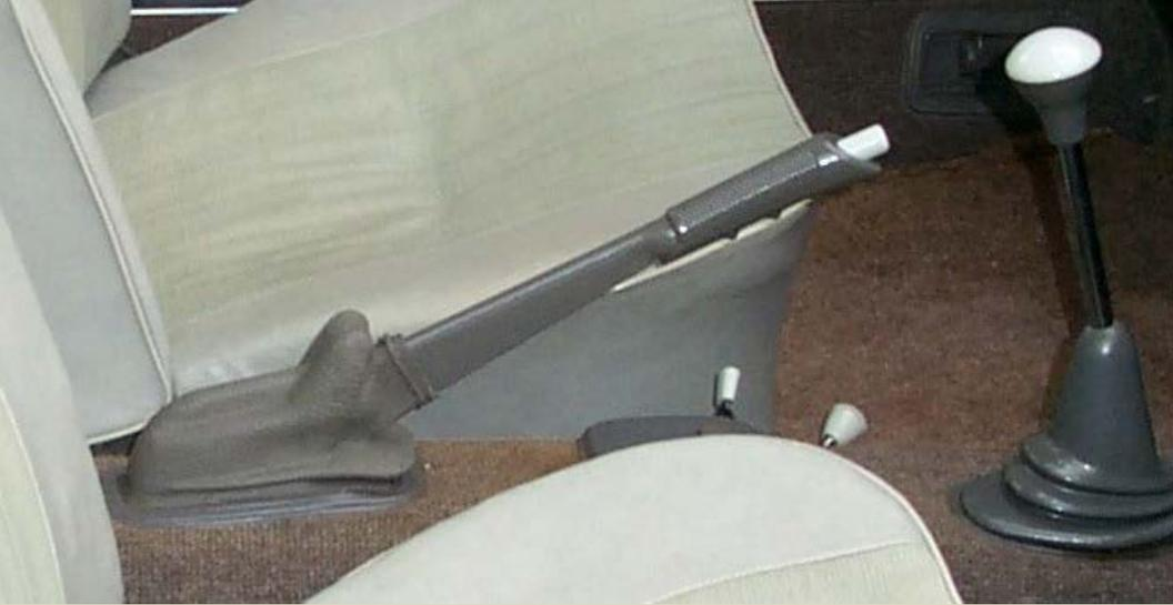
Pedro uses a special Adhesion Promoter clear primer that sticks to the rubber and acts as a primer, allowing the Anthracite paint to be applied better, dry faster, and not crack when the rubber boot is bent during the installation.
