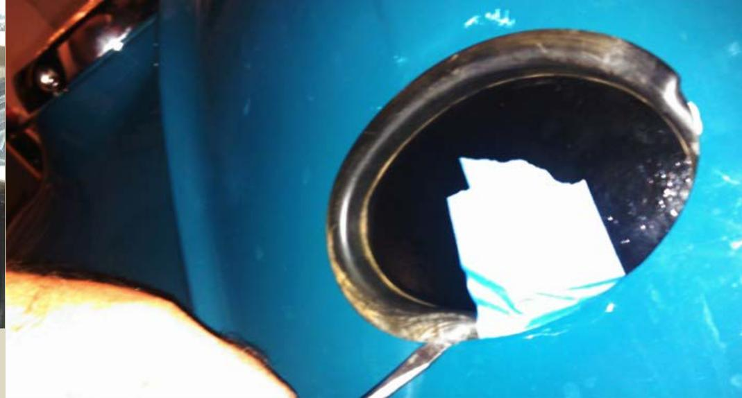
I inserted the plate into the seal and it came out to be 14" (35.5 cm). A box cutter knife blade cut these rubber seals easily. The extra lip on the outer edge was unnecessary so I trimmed it off.
