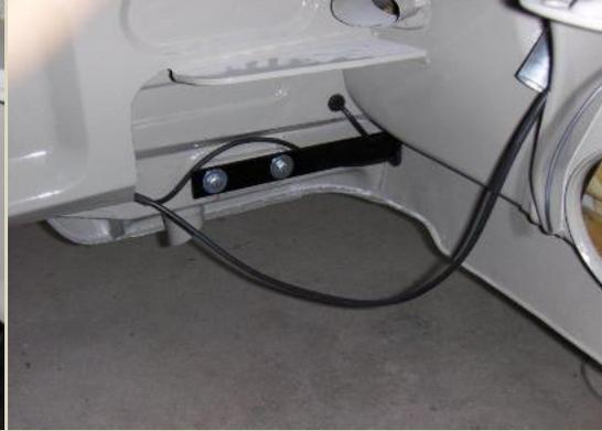
I installed the wiring through the chassis by following the starter wire which goes into the engine bay (pics above). The tach signal wire is the one needed in the engine compartment, which is connected to terminal 1 on the coil. I used the original VW tach installation diagram (below) to get a better idea of how to connect the wires.
