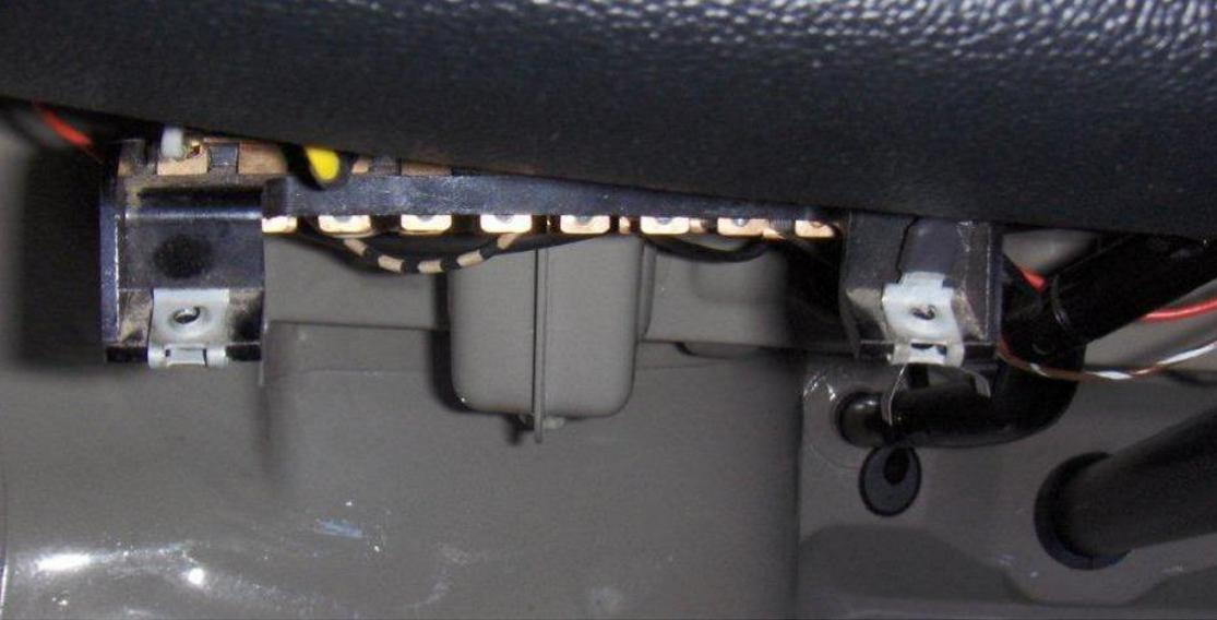
The ground (black wire) from the tach needs to be connected to the grounding terminal clip on the fuse box foot. There's only one clip, so I fitted another one to do the job (above). That allows the tach to have a good grounding when the fuse box is attached to the metal dash panel.
