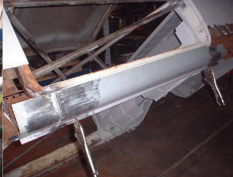
Although the metal tube it runs through was ok, it was easier to bend up a new one rather than sandblast and paint this one. I've found it less interesting doing stuff I've already done but at least it will be easier and in theory quicker this time round.
