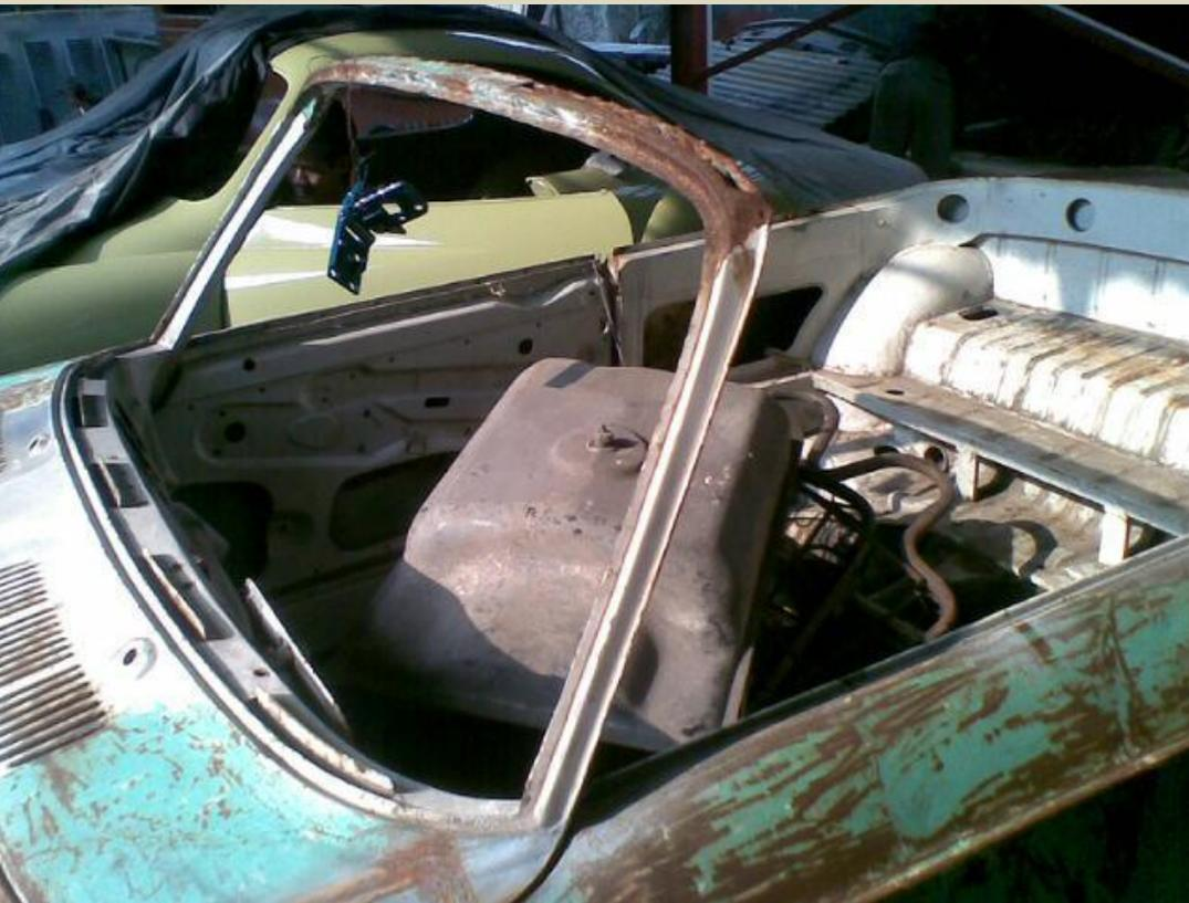
The chassis appears to be solid & original. The strange metal added to the rear window sheetmetal is unique, obviously added as some sort of reinforcement area for the folding top. The original 5-lug rims & brakes are still on the front but the rear has 4-lug rims so there's a bit of sorting-out to be done there.
