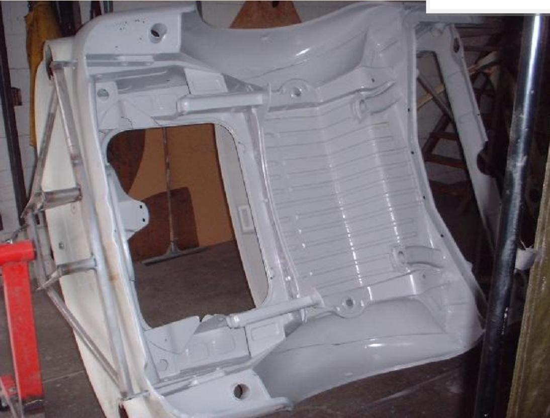
I managed some more cutting last night and opened up the rear fender (below). Most of the bottom section will be replaced with new metal as patching it isn't really a viable option. And while I have a big open hole like this I'll blast and prime the inside of the rear quarter as well.
