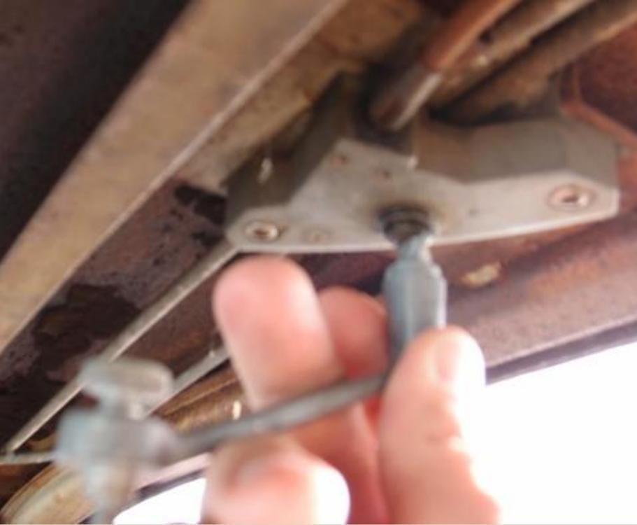
Above: removing the screw to gain access to the crank handle to manually turn the sunroof closed.
