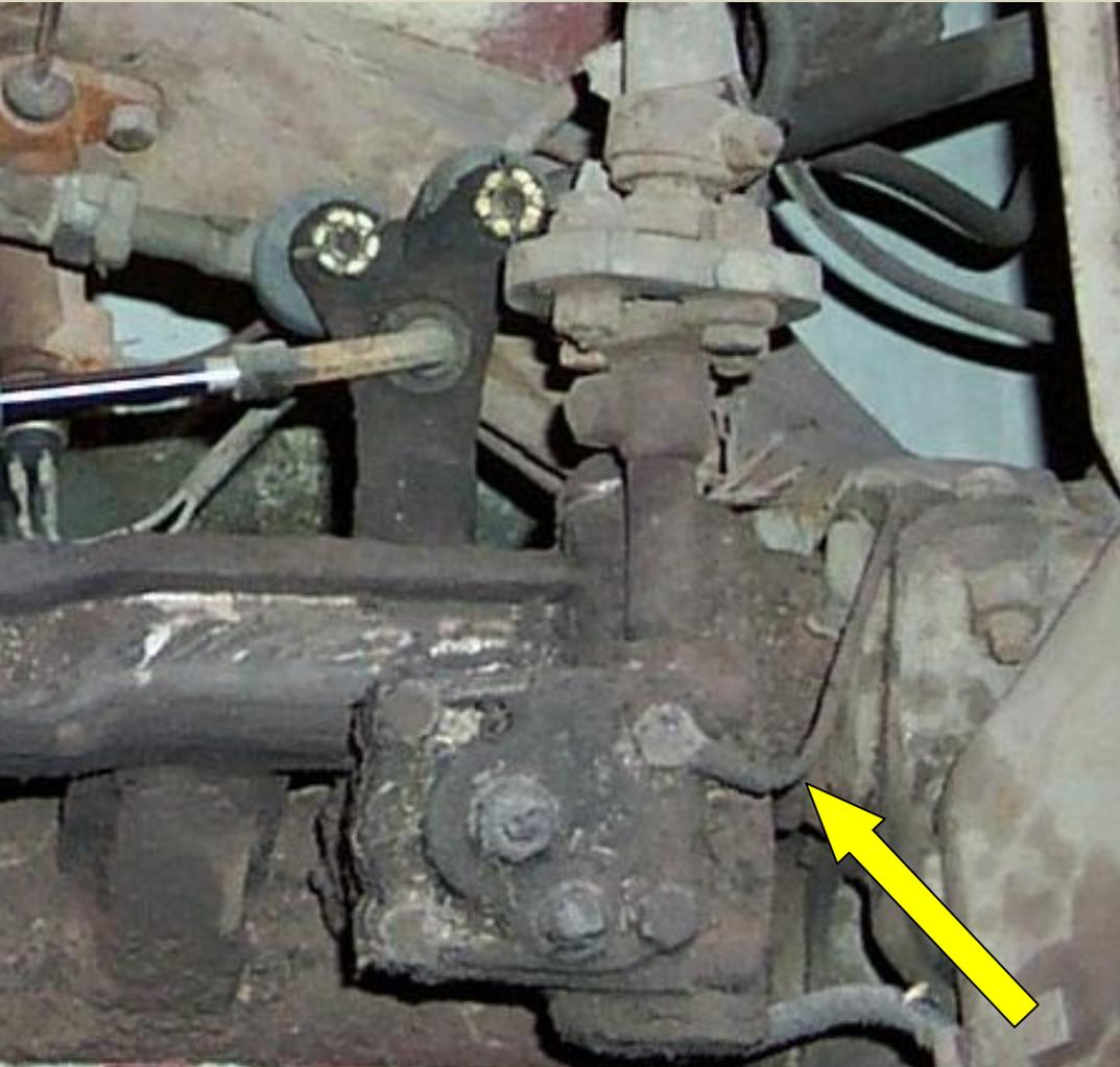
**STEERING BOX CABLE:** The last ground cable is the hardest to access, located on the end of the steering box. It may be easier to access by removing the fuel tank, but that's a lot of work. Smaller hands can get the wire brush up in the tight area to clean the connections and make sure the cable is on tight again. Not easy.
