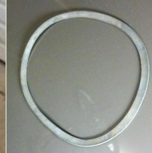
This is an original fog light to body seal. Made from a soft foam rubber, it's a simple flat design on both sides. And it seems so easy to reproduce too.
