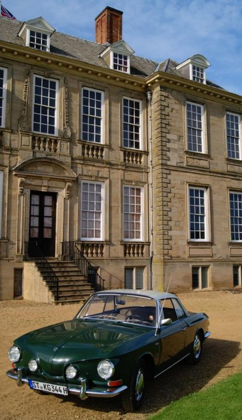
The late-1969 T34 has VIN #349 174 770 and its original 1600cc engine #T 0 645 281, as would be expected with only 33K miles. It was fitted at the Karmann factory with M-Codes 047 dual rear reverse lights, 102 electrically-heated rear window, & 173 textile-belted tires instead of standard bias-ply tires.
